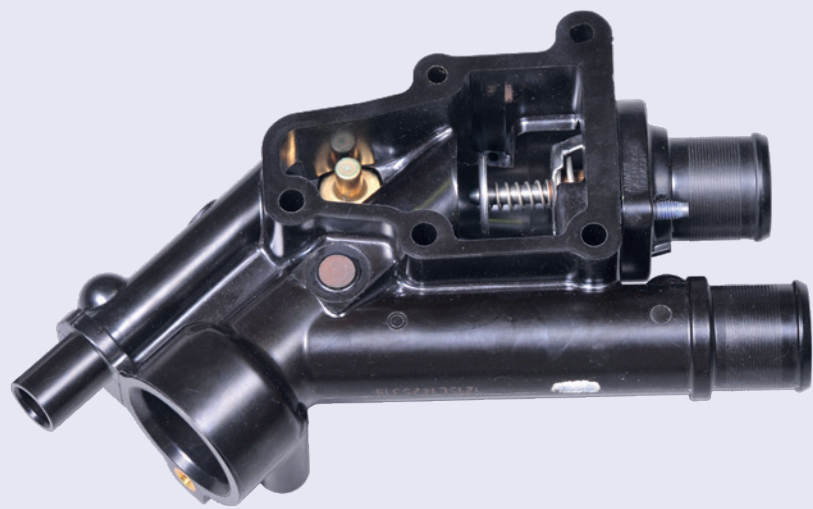
LEFT: THERMOSTAT HOUSING - NEWER MATERIALS USED IN COOLANT CIRCUIT COMPONENTS MUST BE COMPATIBLE WITH ORGANIC COOLANTS BELOW: THERE ARE GOOD AND BAD PUMPS, UNLESS AN IMPELLER IS PROPERLY FORMED AND HAS THE CORRECT RELATIONSHIP WITH THE HOUSING IT WILL CREATE CAVITATION. THIS IS SIMPLE RUST RATHER THAN CAVITATION
